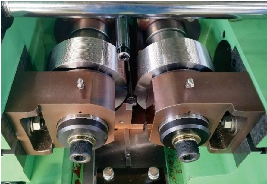
Fig. 8 Appearance of experimental apparatus during DTB-IIC thread rolling
