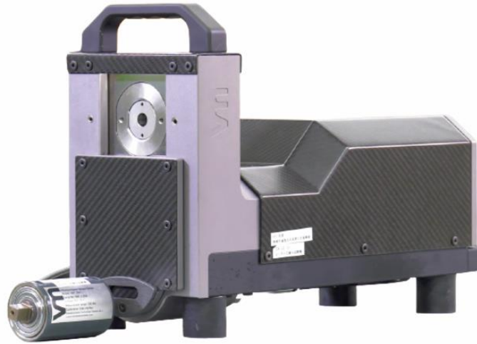
Fig. 13 Junker vibration loosening test bench
